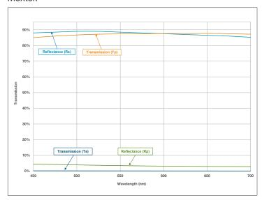
The graphs above show the transmission and reflectance curves for Semrock imaging dichroic beamsplitters and Moxtek optically flat polarizing beamsplitters. Both types of beamsplitter are optimized for use at a 45° angle of incidence.
